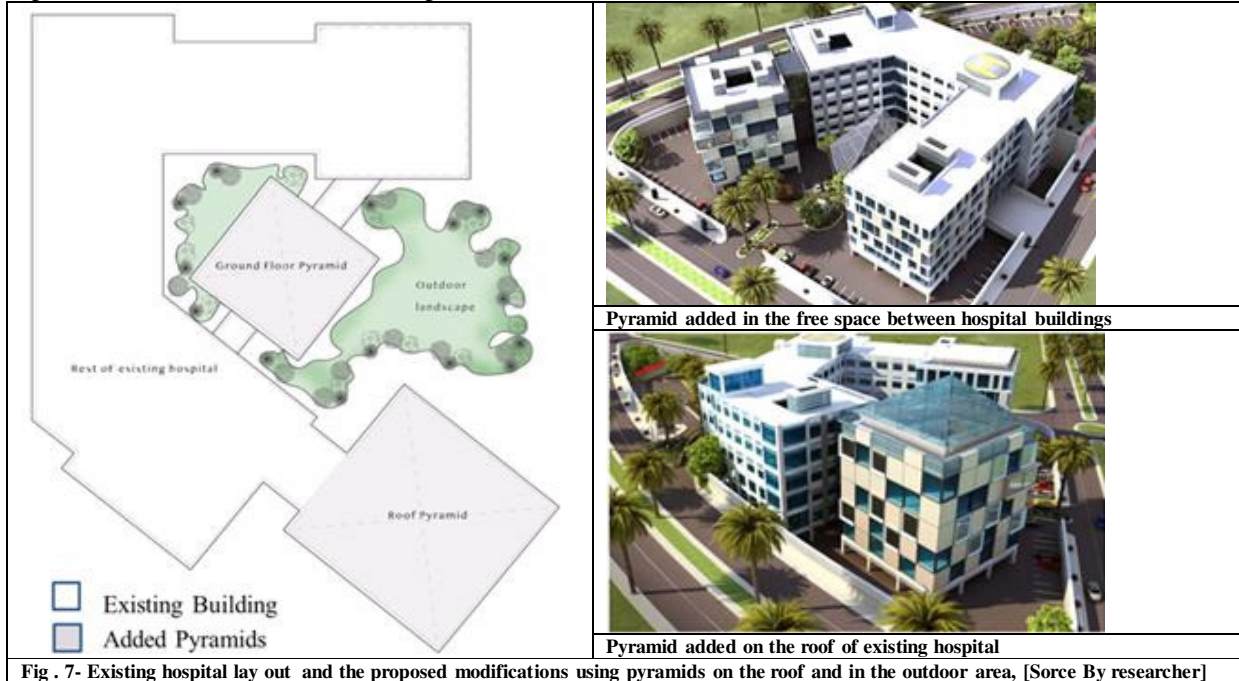
Fig. 7- Existing hospital lay out and the proposed modifications using pyramids on the roof and in the outdoor area, [Sorce By researcher]
