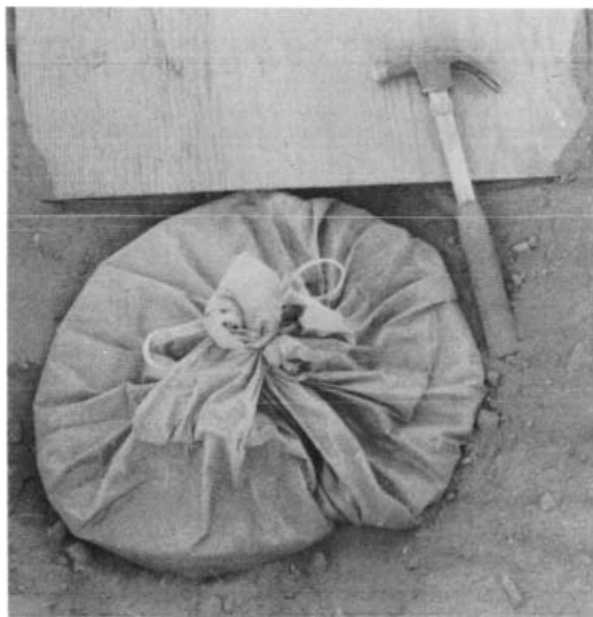
Fig. 8.4. These two 30-gallon polyethylene trash bags, one inside the other, held 16 gallons of water. They were undamaged by 50-psi blast effects while buried in dry, very light soil. The plywood roof and the earth placed over the water bag were removed before this picture was taken.
