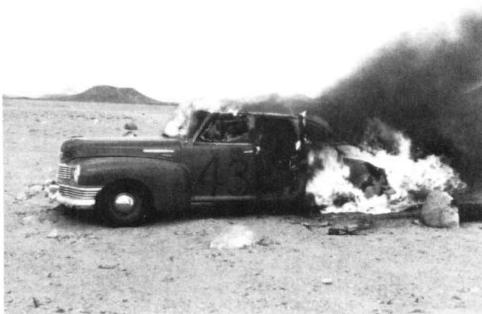
Fig. 7.2. Thermal radiation from a nuclear explosion entered the car above through its closed windows and ignited the upholstery. The windows were blown out by the blast a few seconds later. However, the explosion was at such a distance that the blast wave was not severe enough to dent the car body.
